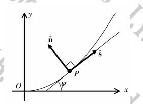
A particle P is constrained to move on a path, so that its distance travelled along that path, measured from the origin O, is denoted by s. The angle the tangent to P at any position on the path makes with the x axis is denoted by  $\psi$ .
