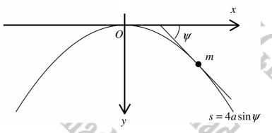
A section of thin flexible gutter type tubing, with a smooth groove running along its length is bend into the shape of a cycloid with intrinsic equation
