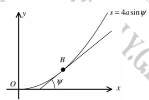
A bead of mass m is made to slide along a smooth wire, which is fixed in a vertical plane, and is bent into the shape of an inverted cycloid with intrinsic equation
