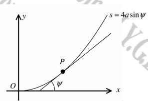
A bead of mass m is made to slide along a smooth wire, which is fixed in a horizontal plane, and is bent into the shape of a curve with intrinsic equation
