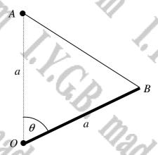
The figure above shows a uniform rod OB of mass m and length a, freely hinged at O, so that the rod can rotate about O in a vertical plane.
