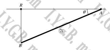
A small light smooth ring is attached to the end A of a uniform rod AB, of mass m and length 2l. The ring is threaded on a smooth horizontal wire. Another small light smooth ring R is threaded on the same wire and a light elastic spring has one end attached to R and the other end attached to B. The system rest is equilibrium with B vertically below R, as shown in the figure above.
