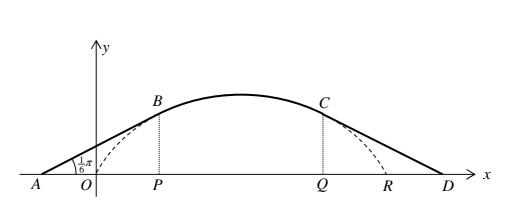
The figure above shows a **symmetrical** design for a suspension bridge arch *ABCD*. The curve *OBCR* is a cycloid with parametric equations
