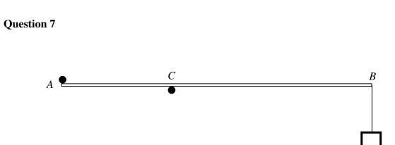
A box of mass 76 kg is attached by a string to one end B of a uniform rod AB of length 5 m and mass 24 kg.
