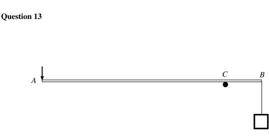
A mechanical lever consists of a uniform steel rigid rod AB, of length 2 m and weight 100 N, placed over a smooth pivot at C.
