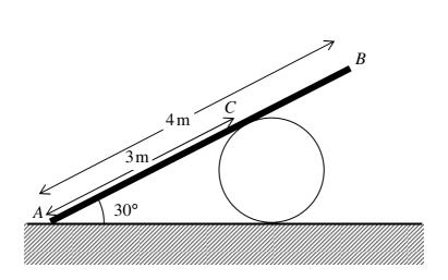
The figure above shows a plank AB resting on a smooth cylinder which is fixed with its axis horizontal to rough horizontal ground. The plank is modelled a uniform rod of mass 10 kg and length 4 metres, resting in equilibrium on the cylinder at the point C, where AC is 3 metres. The end A of the plank rests in limiting equilibrium on the ground, inclined at an angle of 30° to the horizontal. The points A, B and C lie in a vertical plane which is perpendicular to the axis of the cylinder.
