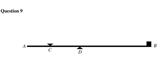
The figure above shows a uniform rod AB of length 1.8 m and mass 3 kg, held in a horizontal position by two small smooth pegs C and D.
