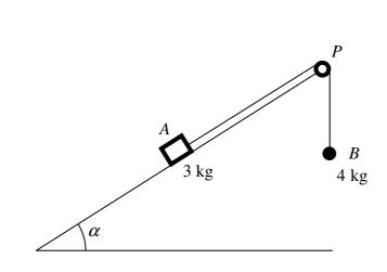
Two particles A and B, of mass 3 kg and 4 kg respectively, are attached to each of the ends of a light inextensible string. The string passes over a smooth pulley P, at the top of a fixed rough plane, inclined at  $\alpha$  to the horizontal, where  $\tan \alpha = 0.75$ .
