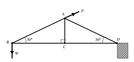
A light rigid framework consists of 5 light pin jointed rods, AB, AC, AD, BC and BD, where |AB| = |AD|, |BC| = |BD|,  $\angle ABC = \angle ADC = 30^\circ$  and  $\angle ACD = 90^\circ$ , as shown in the figure above.
