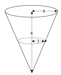
The figure above shows a particle on the rough inner surface of a hollow inverted right circular cone of radius 6 m and height 8 m, whose axis of symmetry is vertical .
