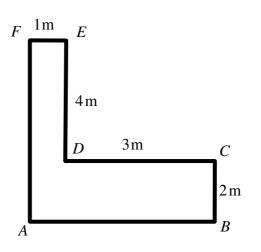
The figure above shows a rigid framework *ABCDEF*, consisting of 6 uniform rods all of equal cross-section and of equal mass density.
