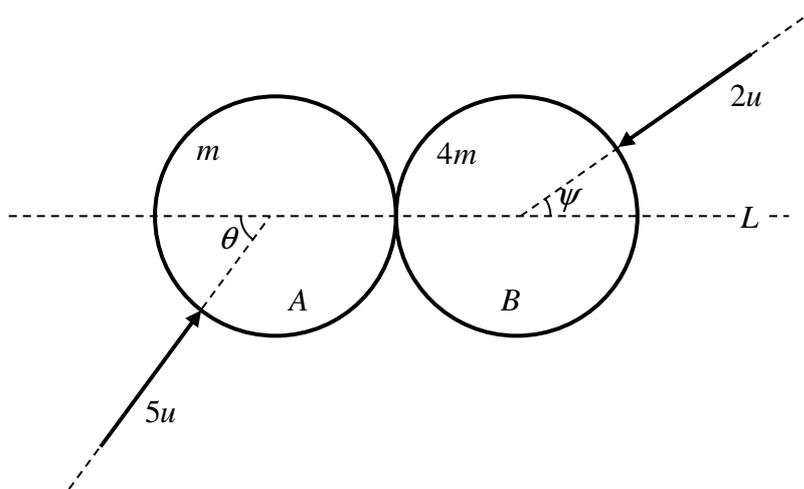
Two smooth uniform spheres  $A$  and  $B$  have equal radii, and their respective masses are  $m$  and  $4m$ . The spheres are moving on a smooth horizontal plane when they collide obliquely, with their centres at impact defining the straight line  $L$ , as shown in the figure above.
