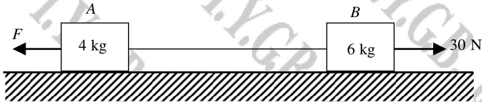
Two blocks  $A$  and  $B$  of respective masses  $4\text{ kg}$  and  $6\text{ kg}$  lie on a smooth horizontal surface and are connected by a light inextensible string.
