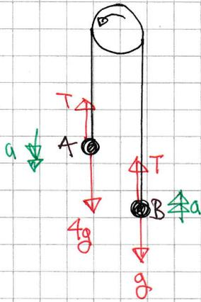
$$\left. \begin{aligned} (A): 4g - T &= 4a \\ (B): T - g &= 1a \end{aligned} \right\}$$
