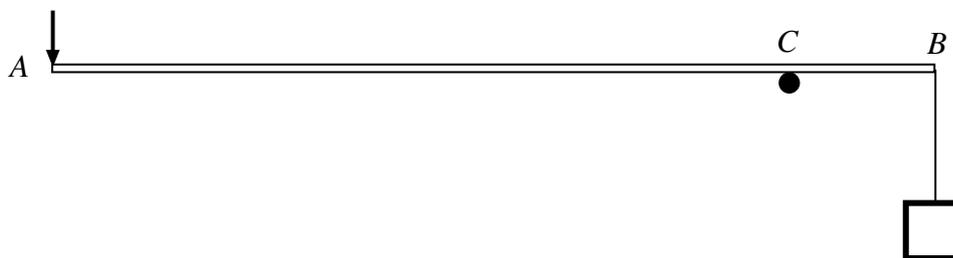
A mechanical lever consists of a uniform steel rigid rod  $AB$ , of length 2 m and weight 100 N, placed over a smooth pivot at  $C$ .
