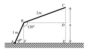
The figure above shows a rigid rod *ABC* where *AB* is 1 metre, *BC* is 2 metres and the angle *ABC* is 120°. The rod is hinged at *A* so it can be rotated in a vertical plane forming an angle  $\theta^{\circ}$  with the horizontal ground.
